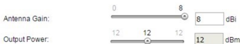
Figure 4.3 Tx Power Setting of EKI-6332GN-AE AP
