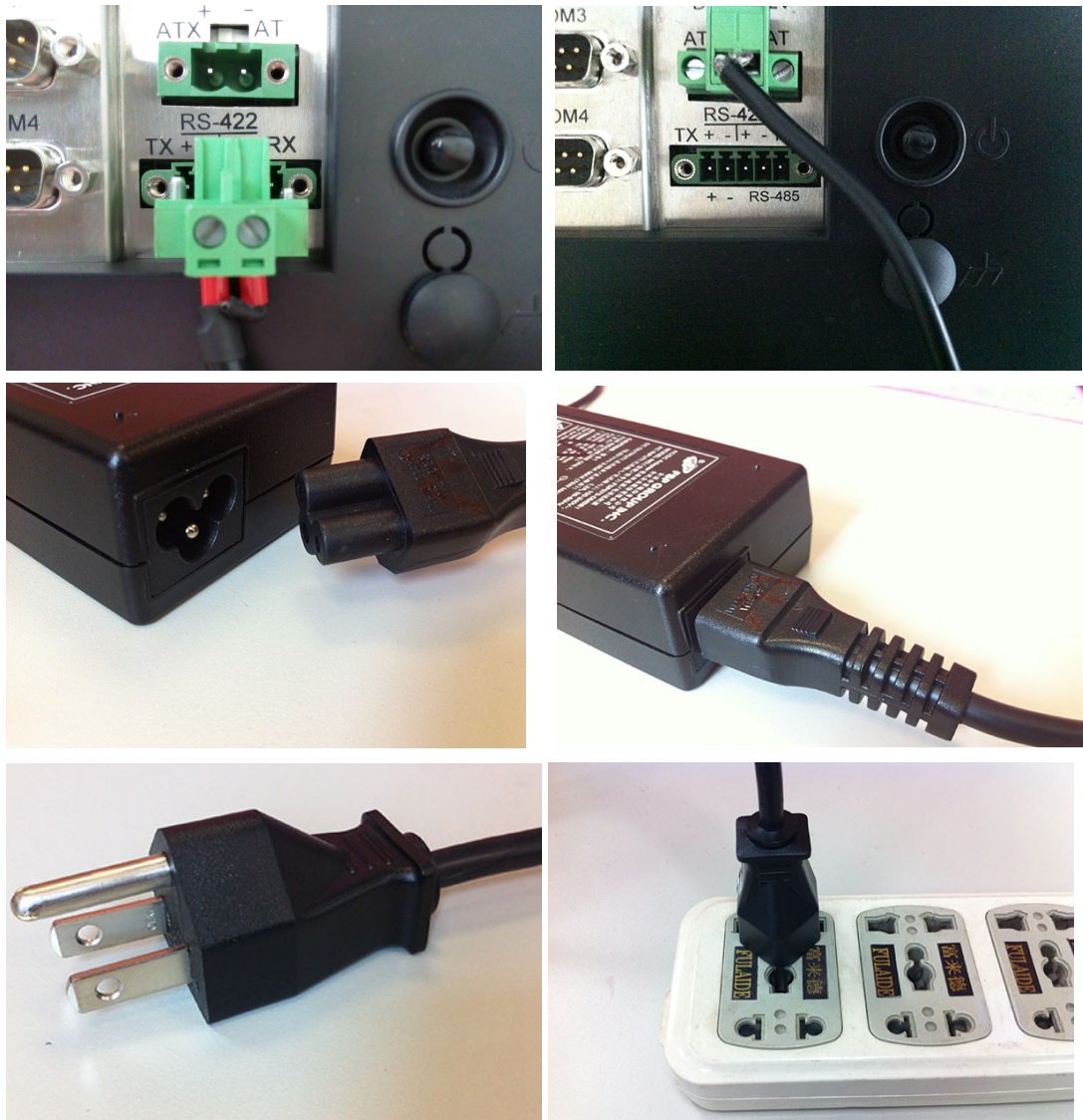
Figure 2.4 Connecting the Power Cable
