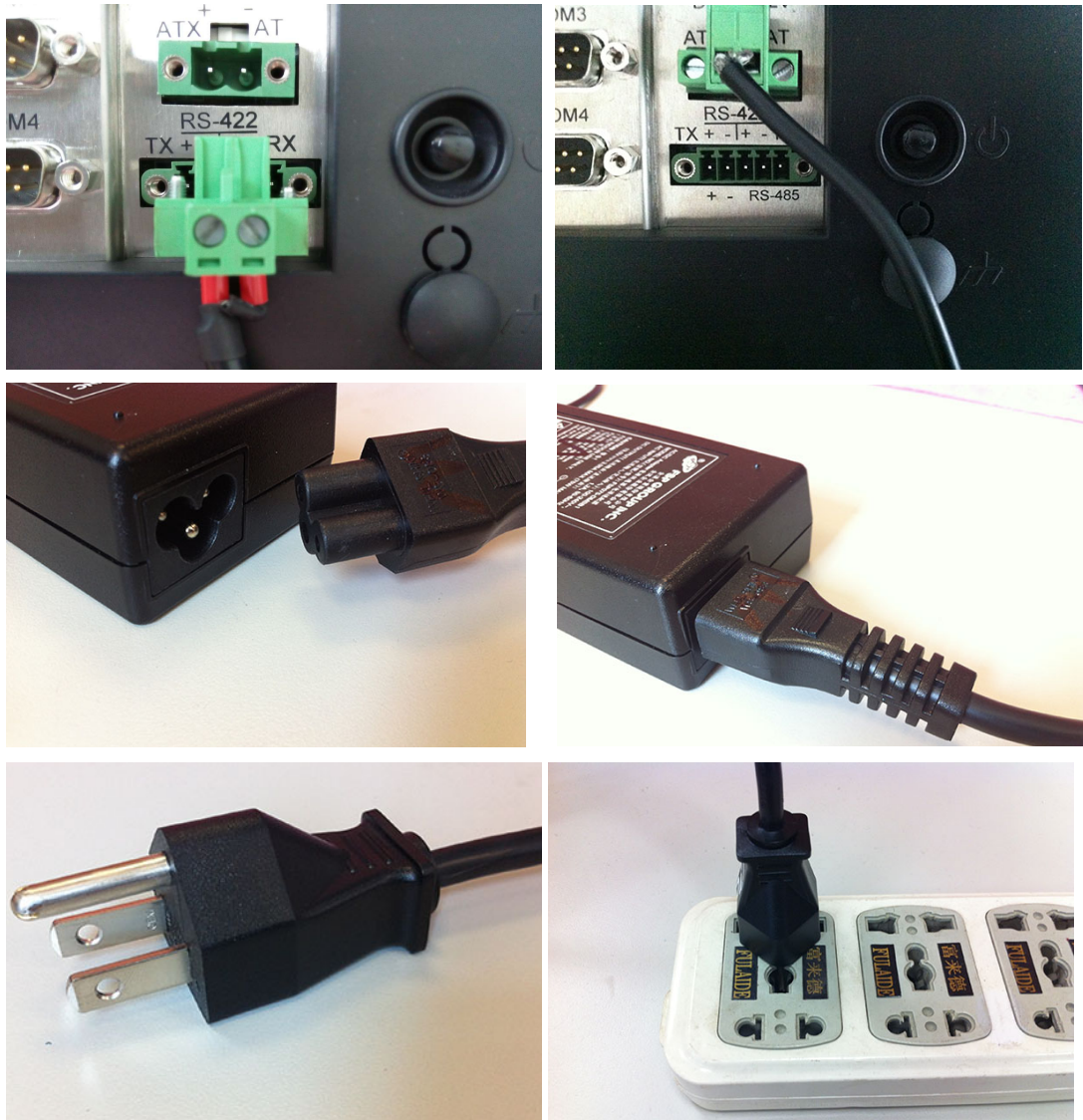
Figure 2.4 Connecting the Power Cable
