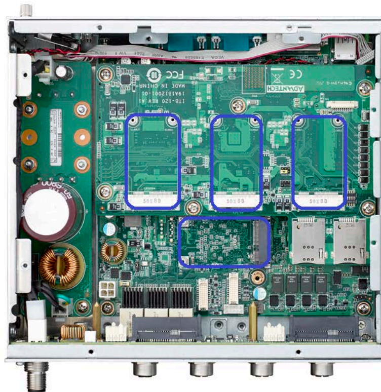
Figure 3.1 Mini PCIe and mSATA Locations on Main Board
